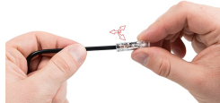
Twist the connector alternately left and right while pulling it off the conductor.
