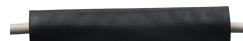
The shrink tube must have an overlap length of at least 30 mm on the cable sheath.
