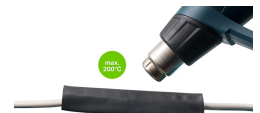
Heat the shrink tube evenly with a hot air blower between 110°C and 200°C.
