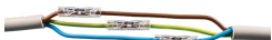
Strip 10 mm conductor per specification and insert connector (example shows staggered connectors).
