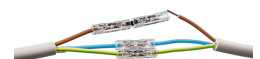
Strip conductor and conductor bridge to 10 mm specified and insert into connector. Only one connector is required for damage points 1 mm.
